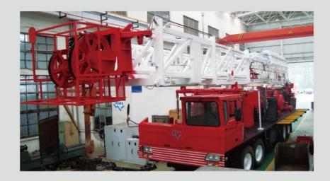
The 5-axle XJ350 is mainly employed under shallow well workover, oil testing, and fishing operations. When a rotary system is employed, this rig can also be used for drilling. TFI offers both workover and drilling options.
